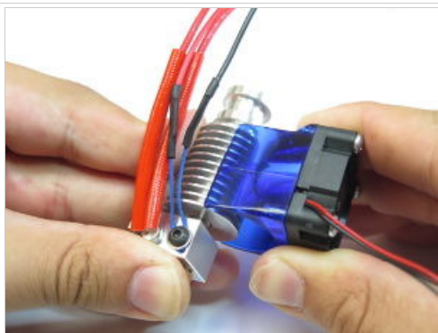
Fan duct clipping to heatsink.
