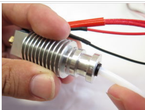
PTFE Tubing being pushed down into HotEnd.
