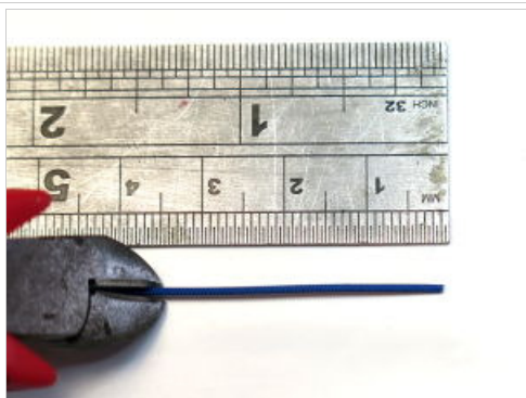
Cutting the sleeving to length. Sleeving on thermistor.
