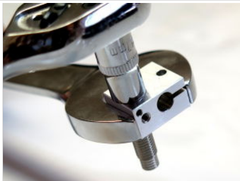
A first, slight tightening of the nozzle against the break.
