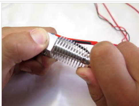
Heatsink is screwed down onto top of heatbreak.
